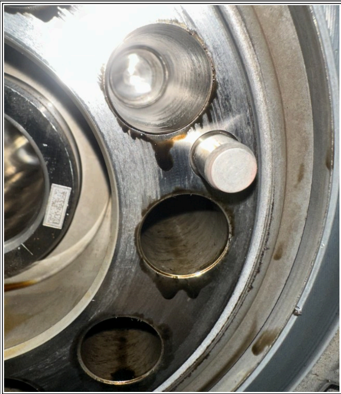
Figure #1: Excess Oil in the flywheel bolt holes
