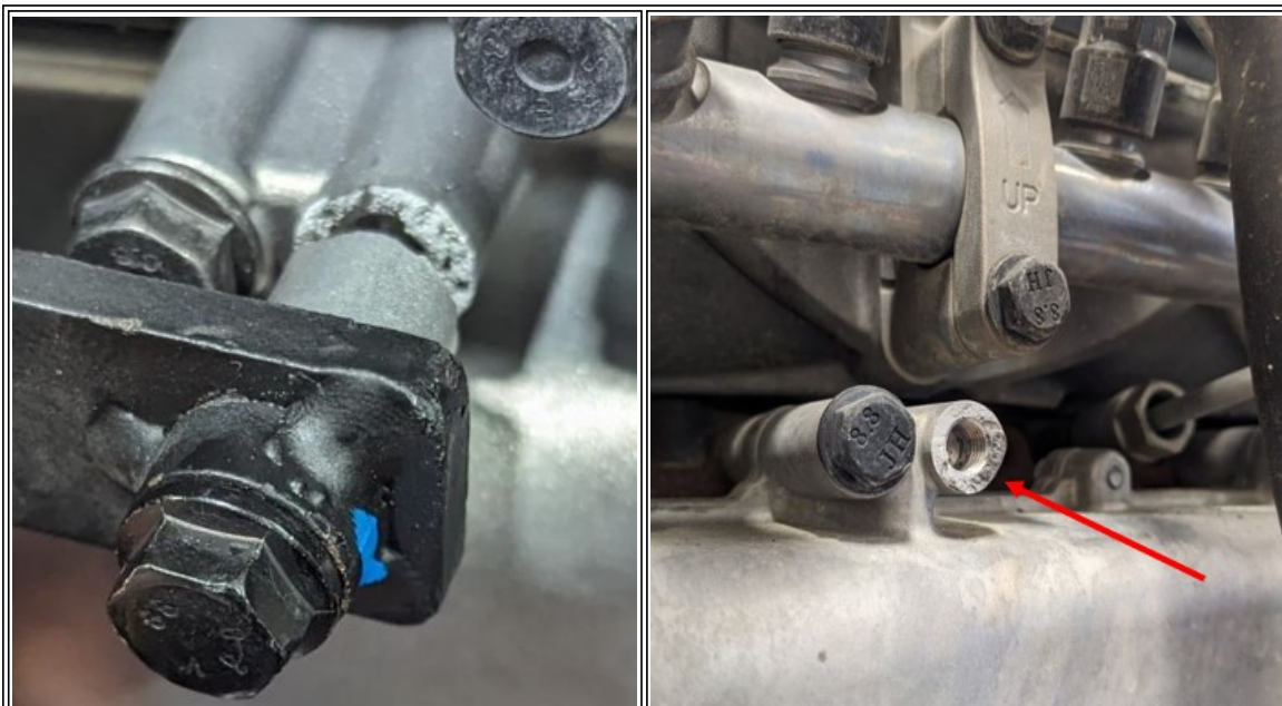
Figure #1: Failed mounting boss
