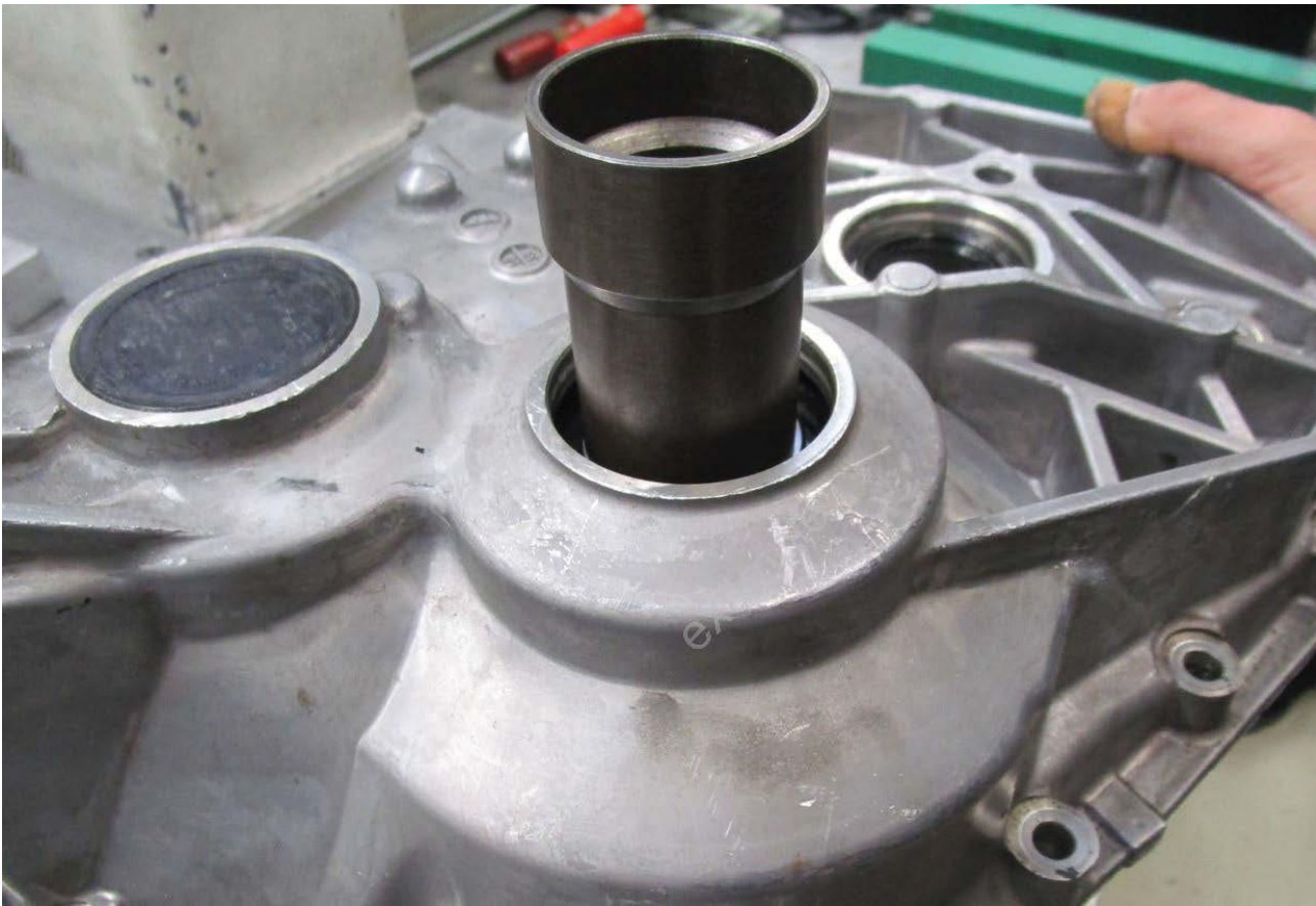
Figure 16. Supporting the inner ring with the thrust piece -VW454- (example).
