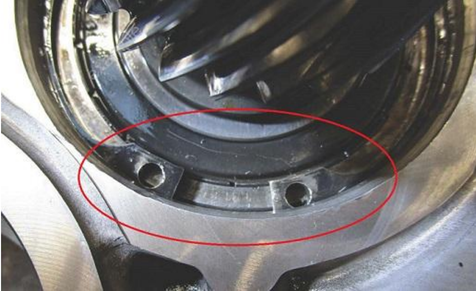
Figure 13. The retaining ring has snapped fully into the groove (example).
