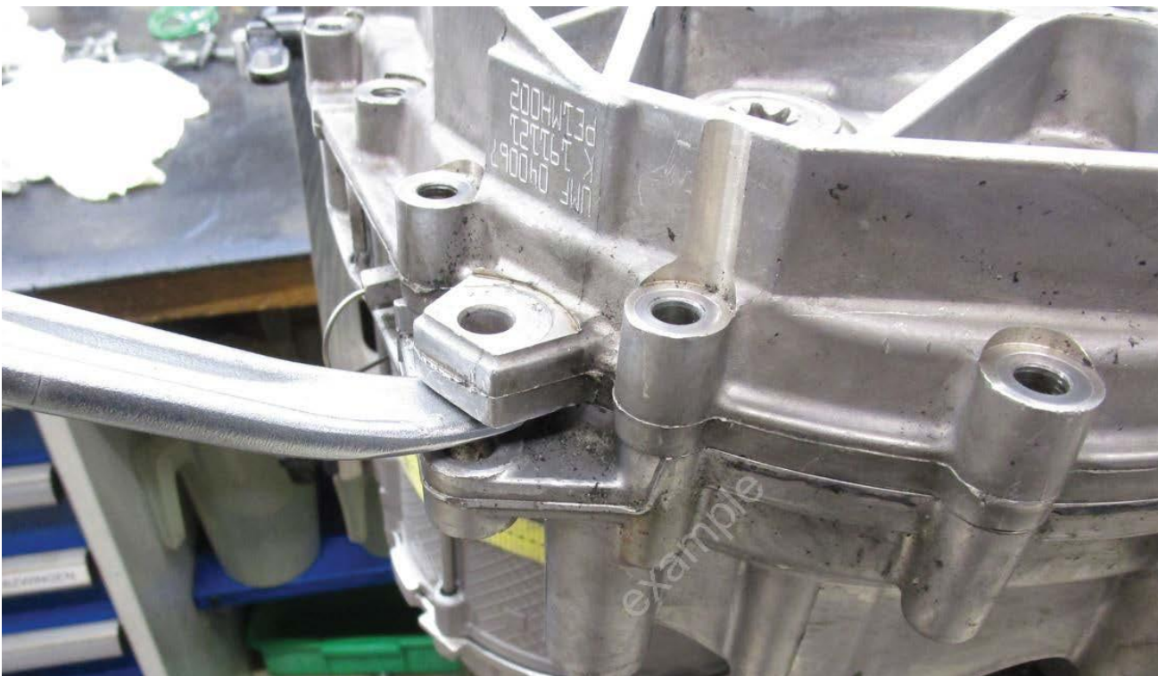
Figure 6. Separating sections of the gearbox housing from each other using the assembly lever.
