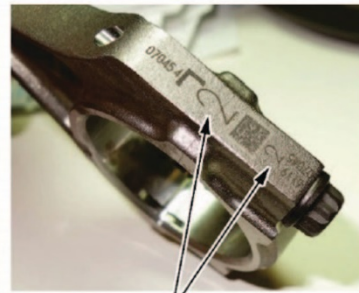
These are manufacturing marks, and do not indicate the cylinder number.
