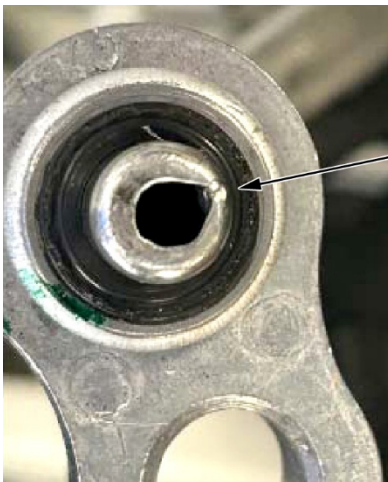
DAMAGED A/C LINE
