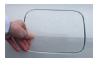
2. Push the fuel/charging door all the way inwards until it reaches the end stop and hold it down.
