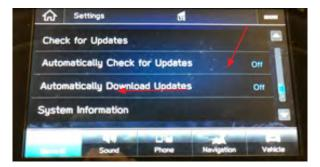
• The currently installed software version will be displayed. If the Software Version is NOT Rel\_UK.25.04.70 (Rel\_UK.YY.WW.70) or later, proceed to Step 2 otherwise no further action is required.
