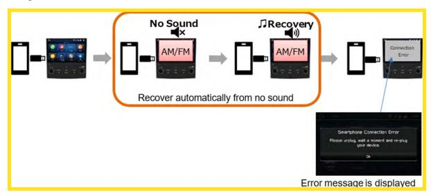
Countermeasure: Re-connecting the USB cable from the iPhone would restore normal operation.
