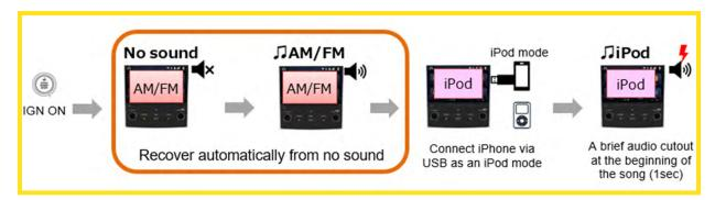
Countermeasure: Turning the ignition OFF and ON.
