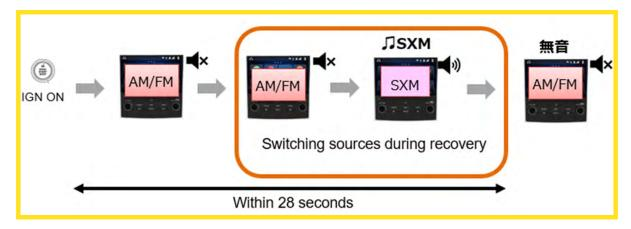
**Countermeasure:** Turning the ignition OFF and ON.
