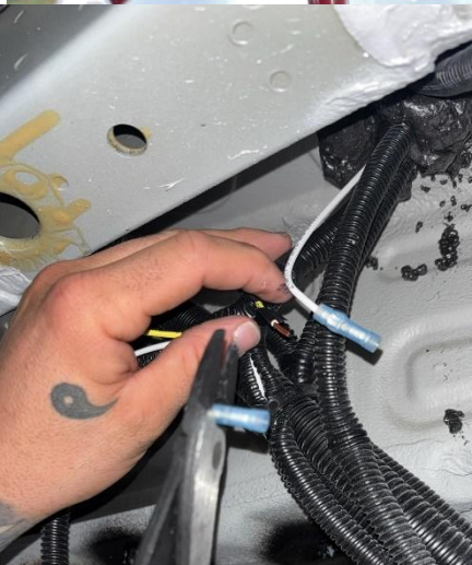
Step 5: cut harness wires back and add butt splices to cap off existing harness
