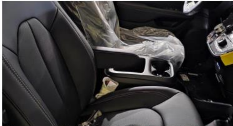
Fig 2: The armrest is horizontal with the seat in design position
