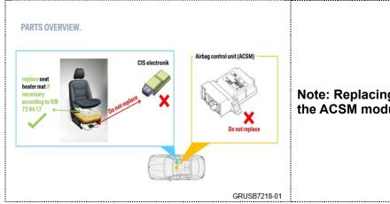
Note: Replacing the CIS electronics and / or the ACSM module will not correct this issue.
