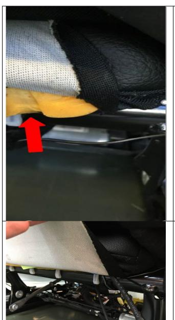
Then place the cable harness back into the groove provided for this purpose in the foam cushion
