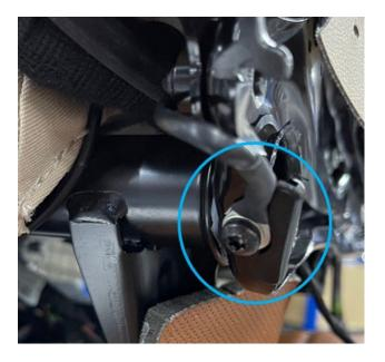
Secure ground screw to eliminate free play to the structure.
