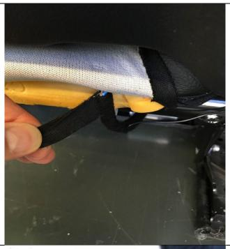
Remove the fabric tape around the wiring
