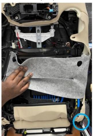
The eyelet on the ground wire should make solid connection to the structure with no free play.
