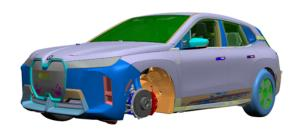
3. Remove the front inner fender liner(s) (highlighted in orange) from the affected side of the vehicle following repair instructions 51 71 039 listed in ISTA/AIR.
