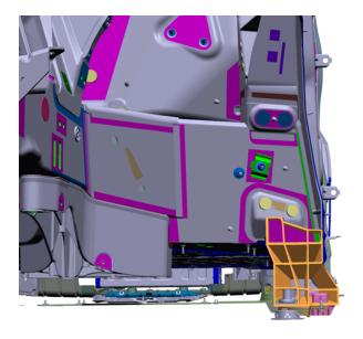
Photo shows the cavities in which the water is trapped (highlighted in orange).
