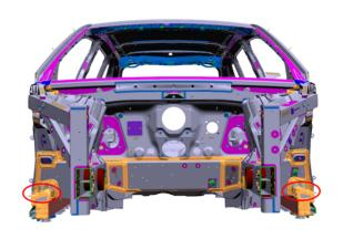
The PVC seam sealer on the front right and/or left inner wheel weld area is not completely sealed (**circled in red**, showing the body shell's firewall and frame rails looking rearwards).
