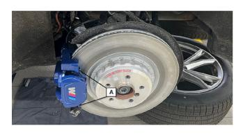
3. Using the approved brake pad paste, PN 83 12 2 296 187 packet (5 ml) or 83 19 2 450 789 8 oz bulk container; apply a small amount to the top and bottom of both rear caliper carriers in the area shown in the photo.
