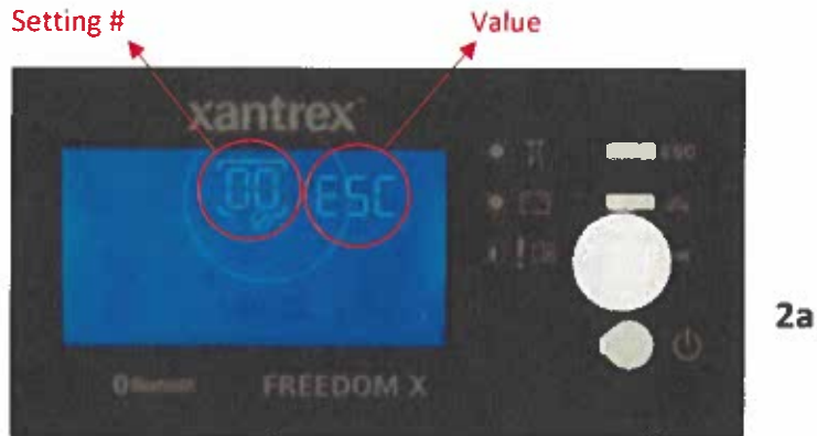
Tiffin GH Setting Codes and Values for Xantrex XC 2000-W and XC Pro 3000-W Inverter
