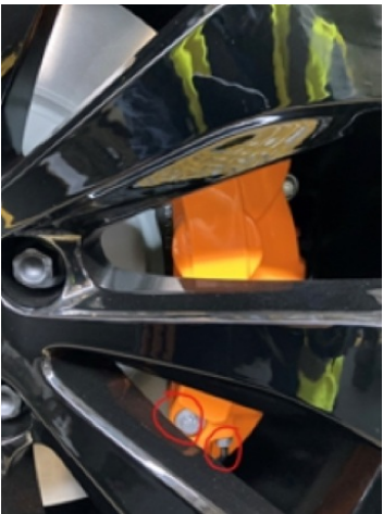
Rear Brake Caliper without Colour-Coded Fixing and connected line ( Normal Condition )
