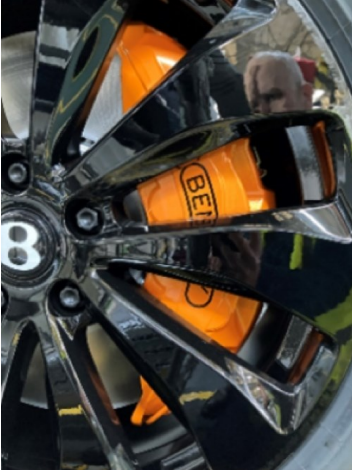
Front Brake Caliper with Colour-Coded Fixing and connecting line
