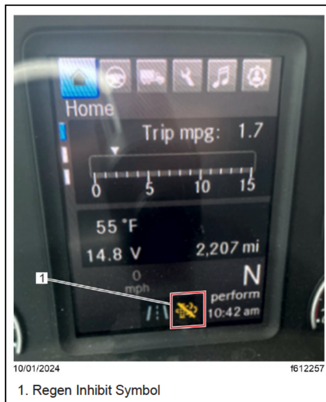
Fig. 14, Regen Inhibit Symbol on the ICUC Display
