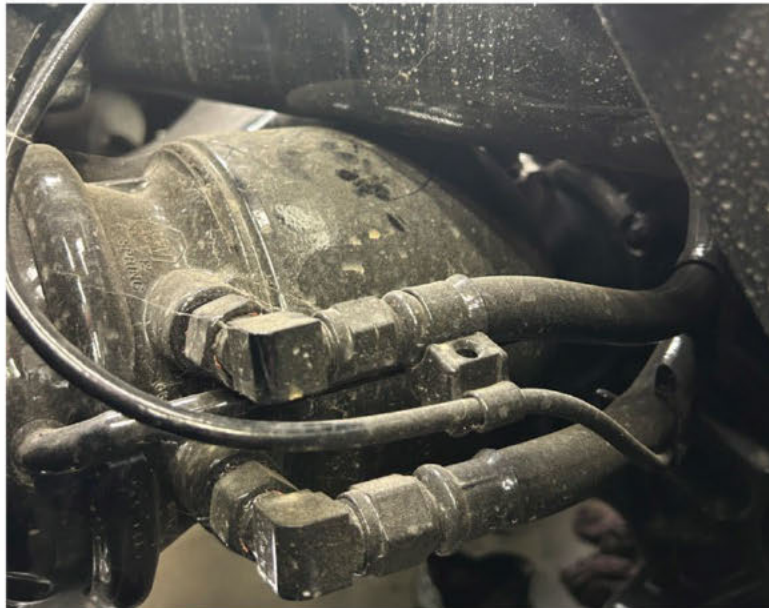
Fig. 2, Frame Contact with the Brake Chamber
