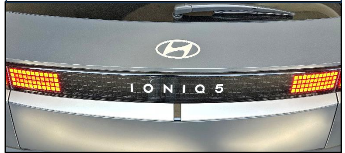
Example of Inside Rear Combination Lamp Working as Designed
