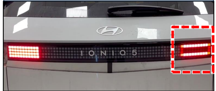
Example of Inside Rear Combination Lamp NOT Working as Designed
