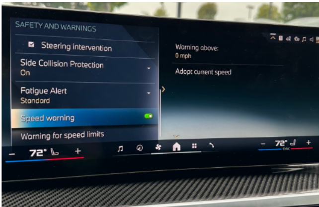
Example photo of the Speed Limit Warning feature and the adopted speed setting discussed in this service bulletin.
