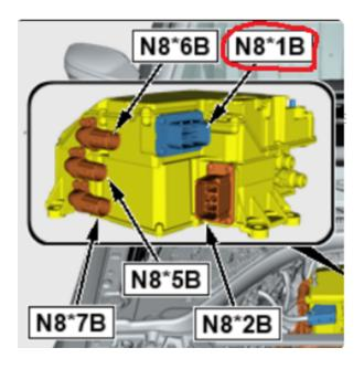
If the pins are found to be faulty, replace the following contact pins 40, 41, 42, 53, 54, 55 for the CCU low voltage (12 V) wiring harness connector (N8\*1B) with pin part number 61 13 6 820 598 (bushing contact MLK 1.2 (0.50 mm²/AG.50 mm)).
