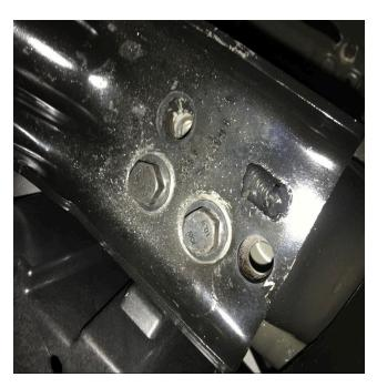
While attempting to unbolt the third-row seat to perform, or to gain access to perform another required repair, one or more of the bolts may not easily loosen. Applying addition force to loosen the bolts may cause the seat anchor body-nuts to break free from their welds.
