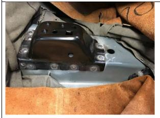
MIG weld the bracket to the support in the drilled holes at the identified spot weld locations.
