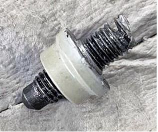
You must cut the bolt to remove the seat.
