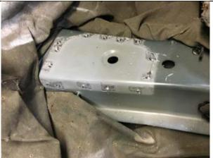
Remove defective bracket by drilling the spot welds and chiseling the defective part from the rear support.
