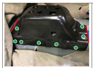
Properly locate new part on the rear support using the scribe lines as a guide and aligning the spot weld positions.
