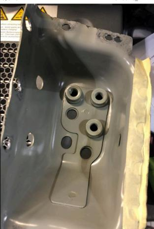
For this situation, replacement of the body bracket with new anchor nuts will then need to be performed so that the third-row seat can be reinstalled and secured.
