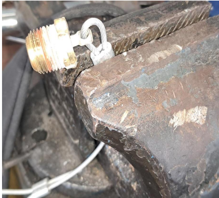
Figure 5- String assembly to the Drain Plug.
