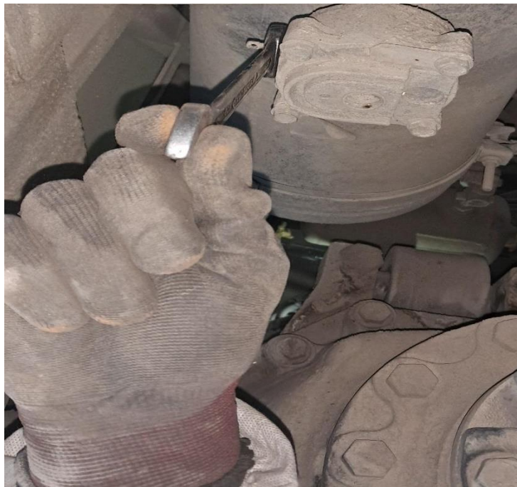
Figure 4- Drain Plugs on the Rear Side must be dismantled with suitable wrench.
