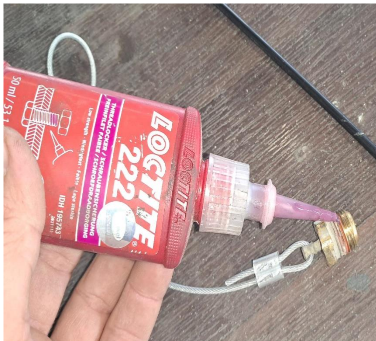
Figure 6 – Before Drain Plugs mounted, must apply Loctite 222
