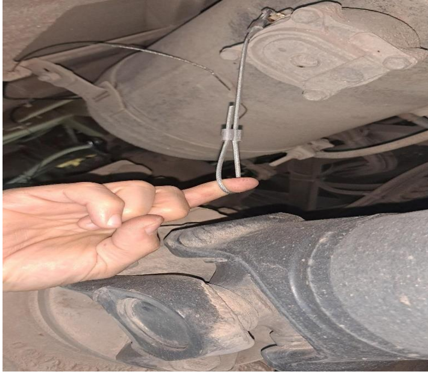
Figure 7- Brake Air Tank's string assembly. Attention! The string must not contact the shaft
