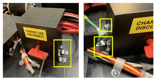
THEN WITH THE BOX PULLED FORWARD, ACCESS THE REAR OF THE DISCONNECT BOX AND REMOVE THE WIRES CONNECTED TO THE INPUT AND OUTPUT POSTS OF THE KEY. KEEP IN MIND WHICH WIRES WENT TO WHICH POSTS FOR WHEN YOU REINSTALL THEM ONTO THE NEW KEY.
