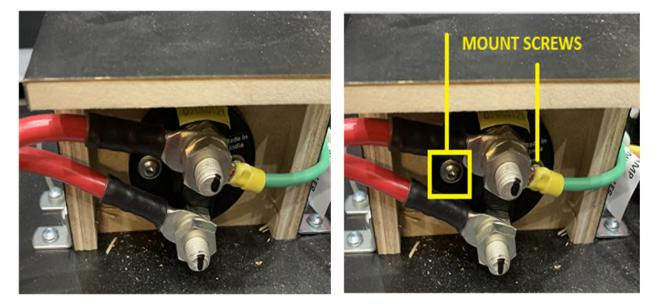
LASTLY, REMOVE THE 2 SCREWS THAT SECURE THE CHARGE LINE DISCONNECT KEY TO THE BACK OF THE BOX. THEN SLIDE IN THE NEW DISCONNECT KEY IN PLACE AND SECURE, HOOK WIRES BACK TO ORIGINAL POSTS AND REMOUNT THE CHARGE LINE DISCONNECT BOX ONTO THE TOP OF THE BATTERY BOX.
