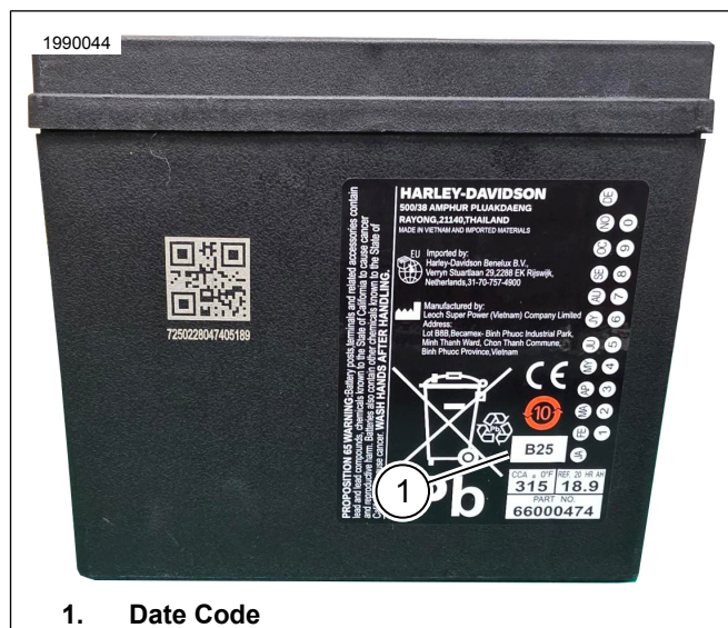
Figure 8. OE AGM Battery Variant
