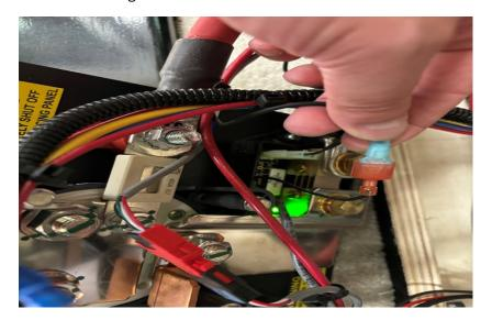
Remove the 2 brass colored bolts using a 9/16 socket. Keep note of the longer bolt as it is required for the connection with the 2 red cables.
