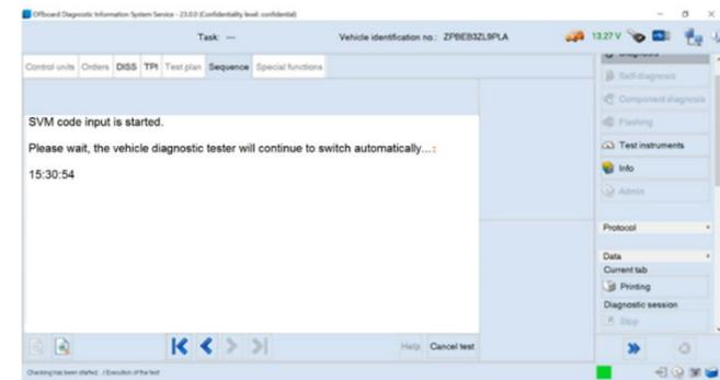
41. The SVM function will automatically continue with identification of the control units in the vehicle.
