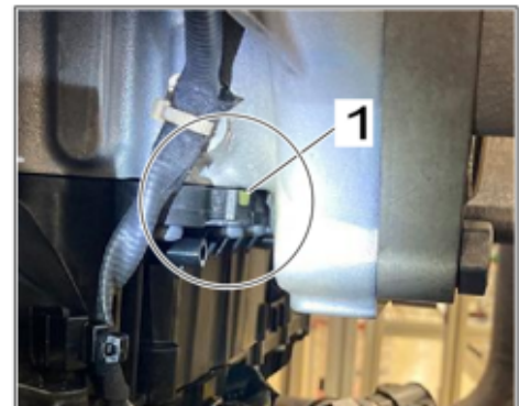
Oil leakage area
