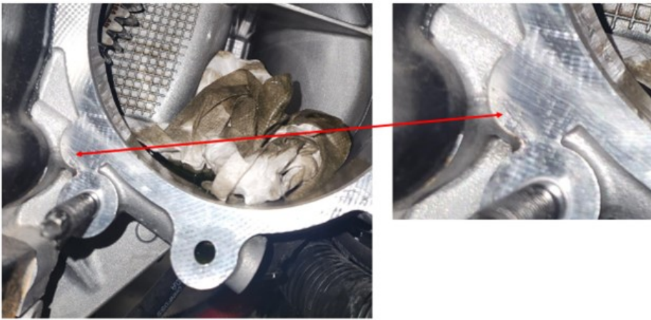
Figure 1 - Gear Housing Boss Leak
