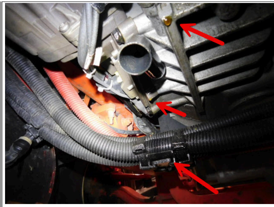
Figure 2 - Oil Leak at the ECA
