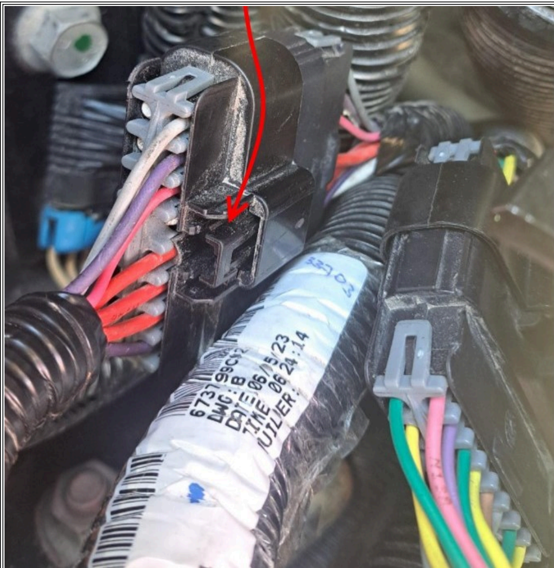
Figure 2: Missing Lock - Connector Pulled Apart
