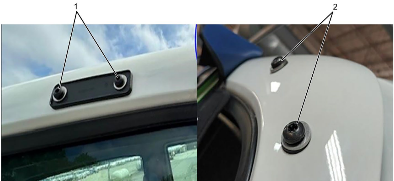
Figure 2. C-Loop Mirror Hardware Properly Installed
