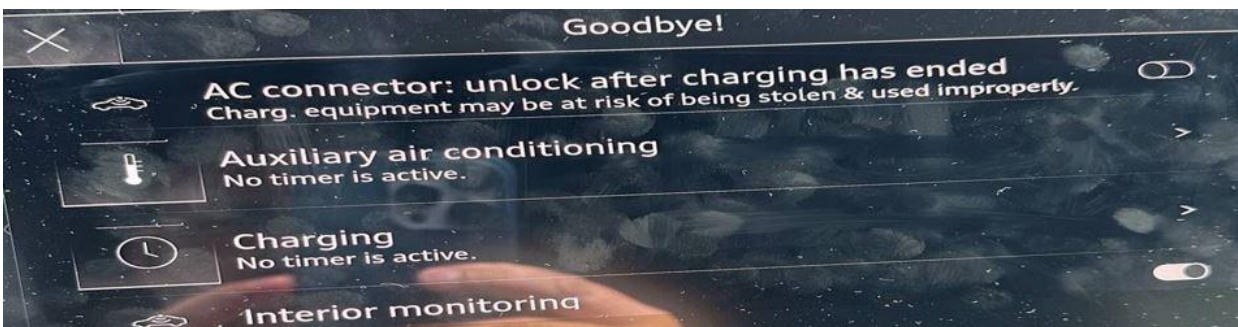
Figure 2: Desired situation - option to automatically release the charging cable at the end of an AC charging procedure is shown in the MMI.
