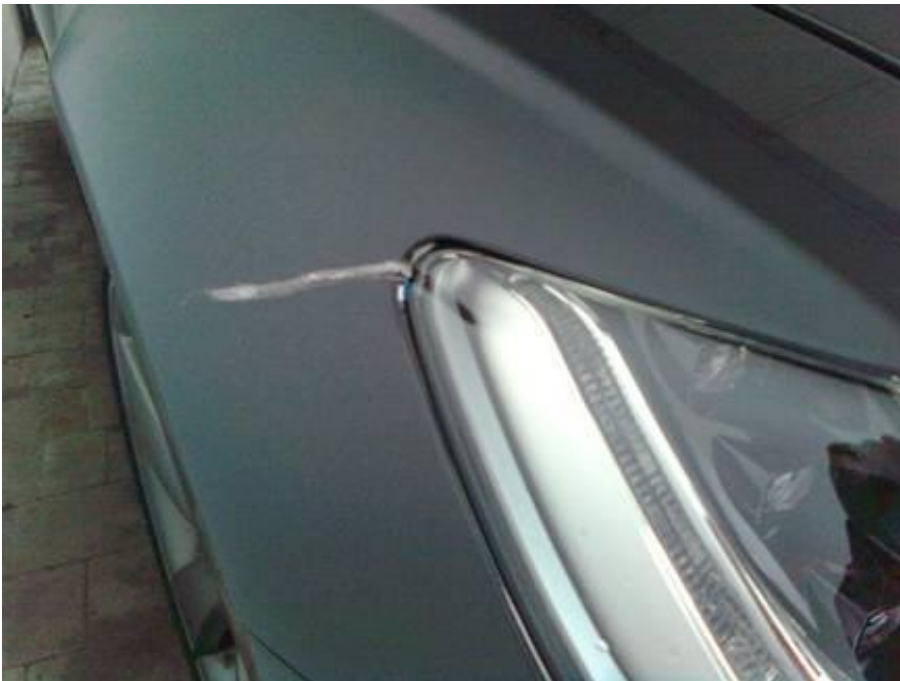
Figure 1. Car wash bristle(s) stuck between headlight and the front fender.
