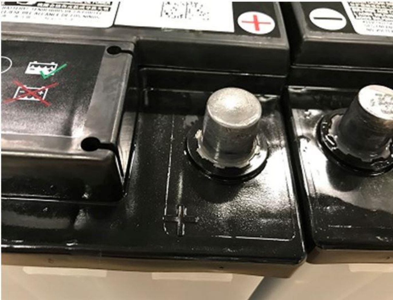
Figure 1. Supplier applies micro-oil as corrosion protection on end terminal and at transition between end terminal socket and cover.
