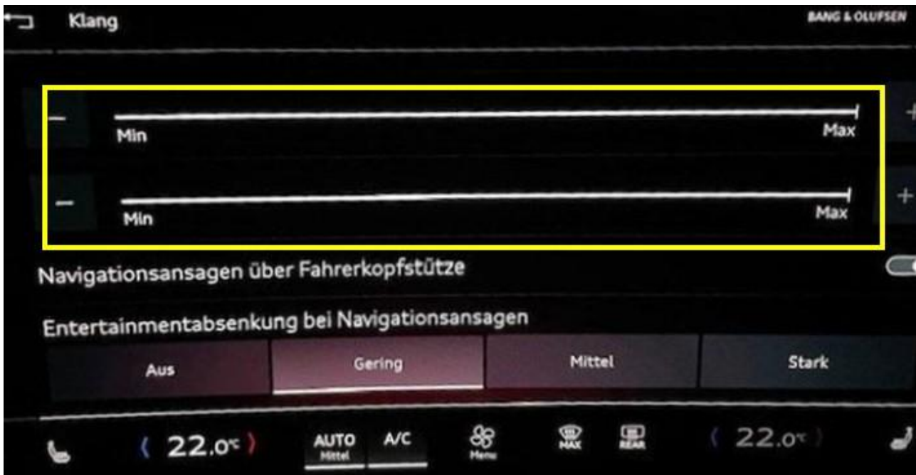
Figure 1. Two unmarked bars are shown instead of buttons for surround sound in the head rests.
