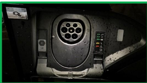
Figure 1. Vehicle with functioning search illumination in the charging flap module.
