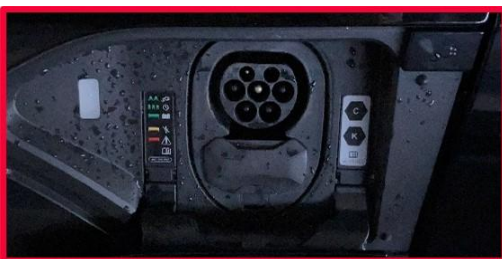
Figure 2. Vehicle with non-functioning search illumination in the charging flap module.
