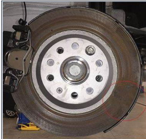
Figure 8: Corrosion, brake pad stuck to brake rotor.
