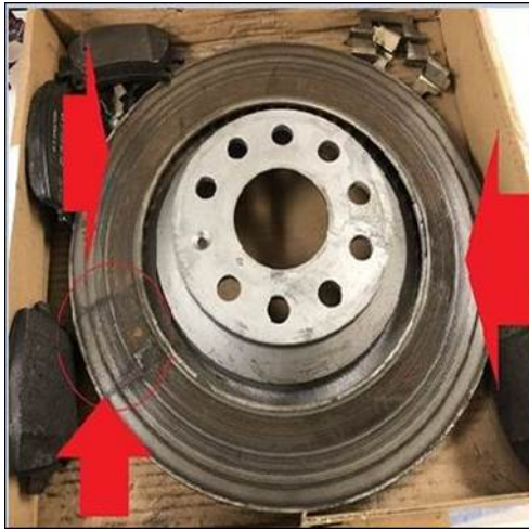
Figure 6: Corrosion, brake pad stuck to brake rotor.
