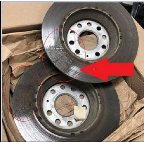
Figure 9: Brake pad stuck to brake rotor
