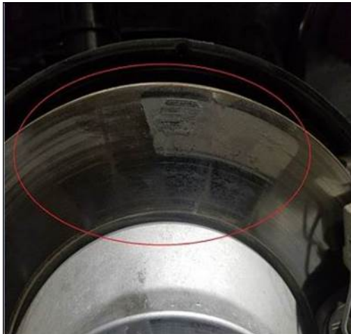
Figure 10: Brake pad stuck to brake rotor.
