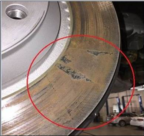
Figure 7: Corrosion, brake pad stuck to brake rotor.
