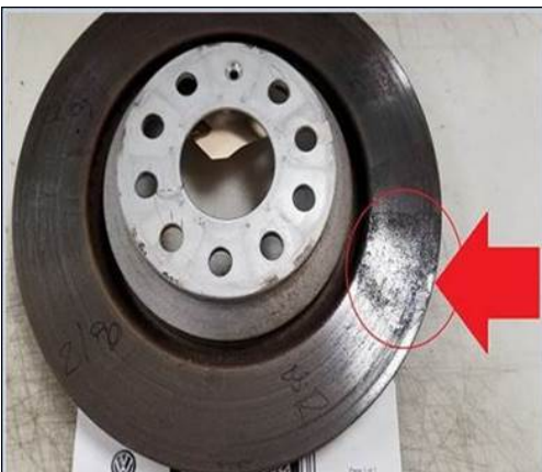
Figure 9: Brake pad stuck to brake rotor
