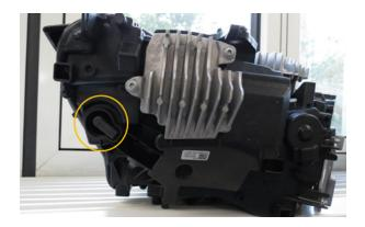
3. Using a suitable tool, remove the outer ventilation grommets from both headlights (circled in yellow).
