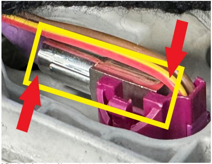
5. This will allow for a release of the excessive tension on the wires and plug connection.
