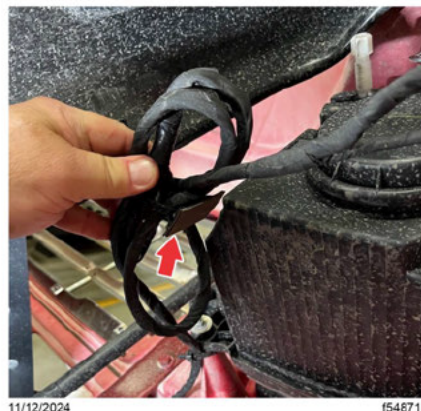
Fig. 2, Stick-On Cable Tie Detached from the Headlight Housing
