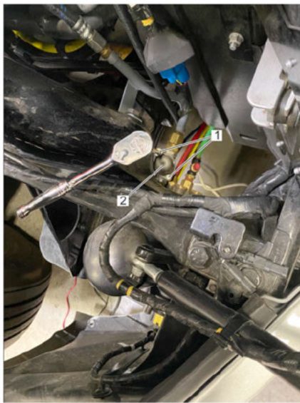
Fig. 1, Removing Bolts of the Overflow Valve
