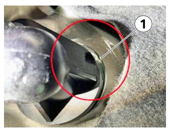
3. With the test plan running (coolant pumps running), use an ultraviolet leak detection light to inspect for coolant leaking around the coolant line connection in the electric motor (1).
