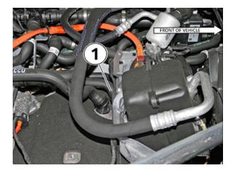
The coolant hose that requires inspection is the lower hos on the motor (1)
