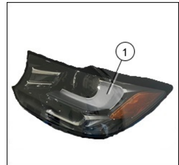
Combination light with AFS (1): Parking light/daytime running light (DRL)
