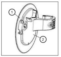
To eliminate this concern, the operation stroke of the fuel-filler lid lock actuator rod has been changed to reduce the play of the actuator rod.
