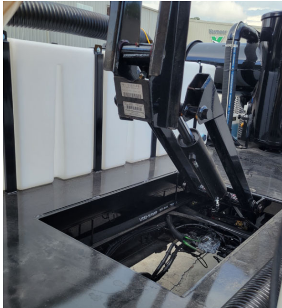
Secure Debris Tank In Upright Position By Stacking 4x4s
