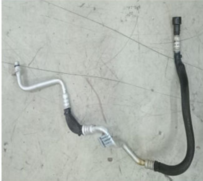
Fig. 3 A/C Discharge Line
