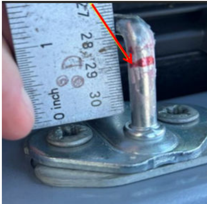
Fig. 2 Striker Spacer Installed
