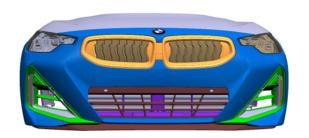
During vehicle assembly, the incorrect kidney grille trim finish (highlighted in orange) was installed.
