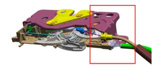
Oxidation/corrosion on the tailgate latch electrical connector and/or mechanical cable.
