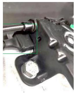
3. If there is a buildup of oxidation / corrosion, with prior customer approval, carefully remove the buildup and install a heat shrink tube around the tailgate latch electrical connector with a diameter or 18 mm and a length of 100 mm.
