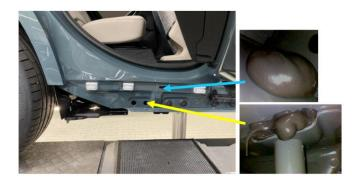
12. After the adhesive has been applied, a curing time of 24 hours is required before moving the vehicle.
