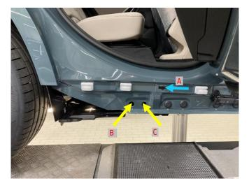
6. Using a borescope, insert the borescope head through **slot A** (blue arrow).
