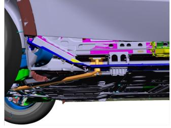
Movement within the mounting bracket (highlighted in orange) that secures the torsion strut to the vehicle's body.
