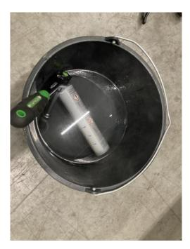
Using filling adhesive (83 19 5 A71 4B0), place the cartridge in boiling water at 212 °F for 10 minutes.
