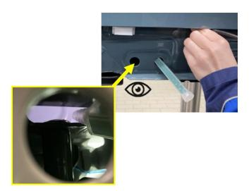
8. Using a mixing nozzle (83 19 2 468 929), insert the mixing nozzle in **slot C** while looking through **slot B**.
