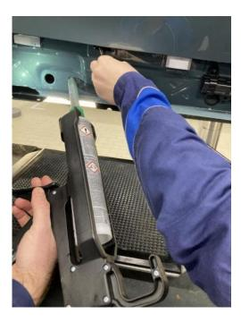
With the borescope head still inserted in slot A, apply the adhesive from both slots B and C at the rate of one quarter of the cartridge.
