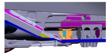
**Note:** The mixing nozzle tip needs to be sitting on top of the mounting bracket (highlighted in orange with the blue arrow).
