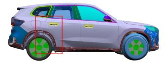
While driving on a smooth and/or uneven road, a "popping" sound is heard from the bottom of the C-pillar area. This can occur on one and/or both sides on the vehicle C-pillars.
