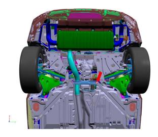
2. On the side of the vehicle from which the sound is generating, remove the rear bolt that secures the torsion strut to the rear axle (red arrow points to the bolt).
