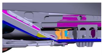
**Note:** The mixing nozzle tip needs to be sitting on top of the mounting bracket (highlighted in orange with the blue arrow).
