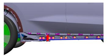
5. Remove the third clip that secures the rocker panel to the vehicles body (red arrow pointing to the clip).
