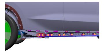
4. Remove the two body plugs (circled in red).
