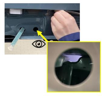
7. Using a mixing nozzle (83 19 2 468 929), insert the mixing nozzle in **slot B** while looking through **slot C**.
