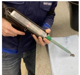
10. Install the mixing nozzle on the adhesive tube and adhesive gun.
